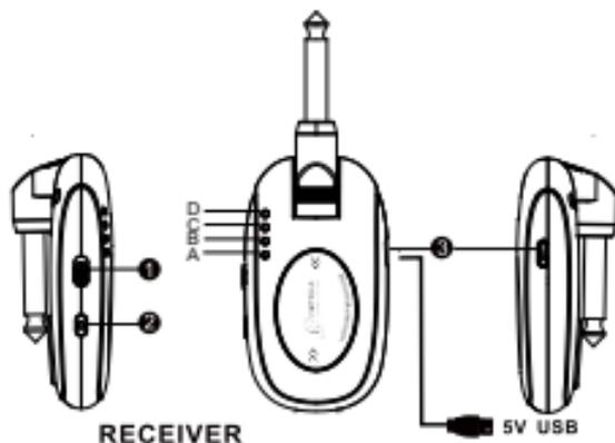
1. **Power** - Slide Switch to turn on/off TRANSMITTER/RECEIVER
