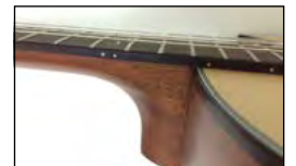
14th fret heel to body connection
