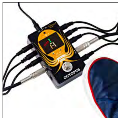
Power plant for 8 devices
